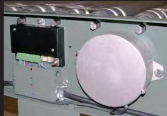
E24™ is a brushless, gearless, low RPM, high torque motor, designed specifically for driving conveyor rollers reliably and efficiently. The external motor approach to 24 VDC technology provides exceptional flexibility, superb heat dissipation, and a robustness that cannot be achieved with motors embedded in conveyor rollers.
