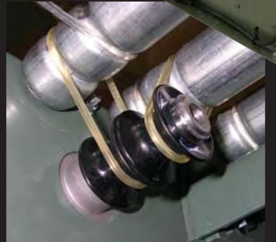
By replacing the drive spool with the optional limited slip spool assembly, E24™ conveyors can be used in minimum pressure applications. No other 24 VDC conveyor drive technology offers this unique capability.
